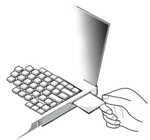
14. Slide the CardBus Adapter completely into the PCMCIA CardBus slot. When the CardBus Adapter is properly inserted, Windows NT finds the new hardware and a beep is emitted that indicates that installation is complete.
